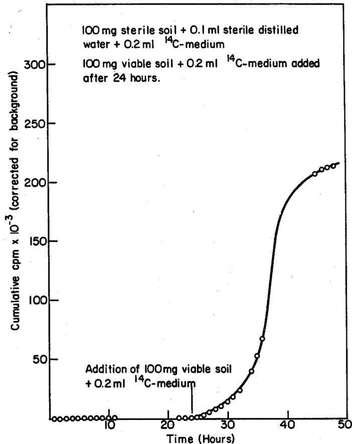
Fig. 11. Reuse of chamber for positive response following initial negative test.
