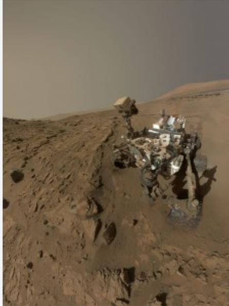
Curiosity self-portrait at "Windjana" drilling site. The Mars rover used the camera at the end of its arm in April and May 2014 to take dozens of component images combined into this space-based selfie.
